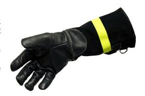
The structural firefighting glove is EC marked proving the approval to sale according to Council Directive 89/686/EEC. This PPE belongs to 3<sup>rd</sup> category in conformity to EN 659 - EN407 PROTECTION CLASSES 4231XX - EN 388 PROTECTION CLASSES 2244.
