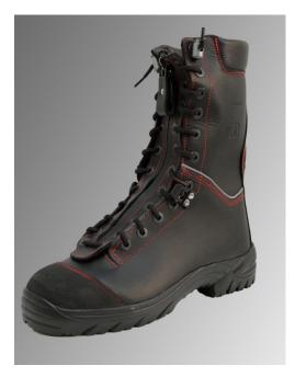
The upper is made of: one piece vamp, linked to a 2 quarters by means of a triple stitching; a back stripe joined by triple seam to the vamp and the quarters; a collar made of veal leather; a bellows tongue. The boot height as measured from the heel base to the collar top is 250 mm +3%, in size 42. (all other sizes develop total height harmonically).
